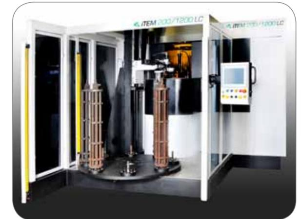
The rotary indexing table is equipped with 8 stations, the deburring fixtures and the workpieces are placed on it and hydraulically driven towards the machine. One fixture at a time is lifted into the machine and placed on the closing plate by the gripper.
