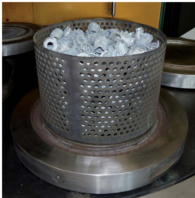
Cage with bulk goods for the deburring chamber \varnothing 400 x 300 mm
