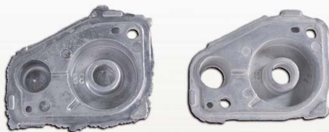
Zinc diecasting part before and after TEM
